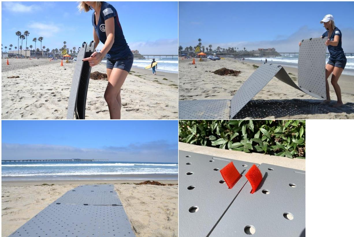
**To secure a hinge**, simply place one end through a panel hinge slit with the hook (rough) side facing up, and thread through the corresponding hinge slit on the opposite panel (see image above, right). Leave approximately 1/4 of an inch gap between panels when hinged together to
